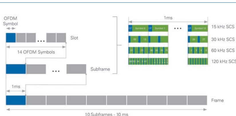
Figure 6: NR frame structure
