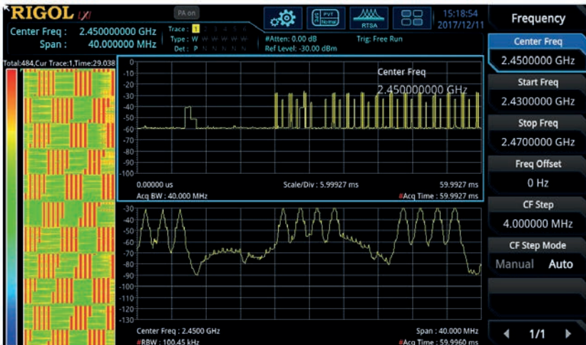
Figure 11: Normal trace vs spectrogram vs PvT of a Bluetooth signal
