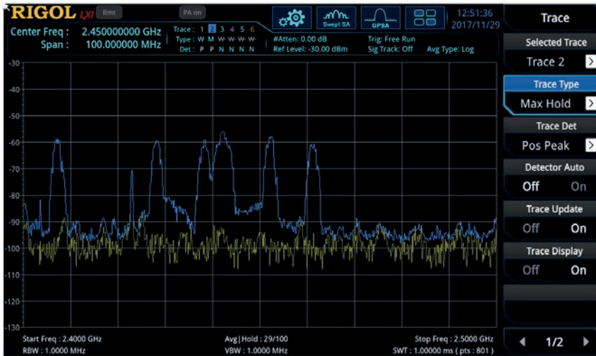
Figure 2: Bluetooth signals are only visible via the SA's maximum hold function
