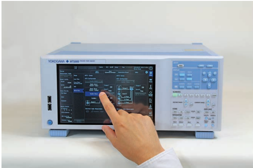
Figure 3: A Yokogawa WT5000 is configured for simultaneous synchronised measurements from four torque and rotation sensors to determine the overall efficiency of four motors
