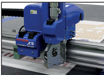
Tape dispenser tool allows adhesive tape to be automatically applied to finished jobs.
