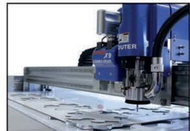
Powerful router easily cuts a wide range of signmaking substrates to a high quality finish.
