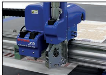
Tape dispenser tool allows adhesive tape to be automatically applied to finished jobs.
