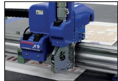
Applies a range of adhesive tapes direct to substrate during cutting process
