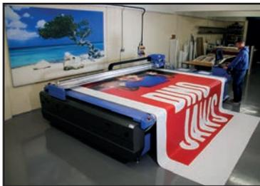
Conveyorised machines enable continuous processing of flexible roll media
