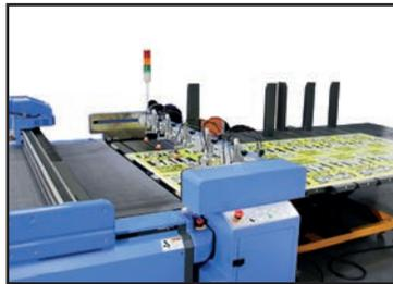
Automation options such as sheet feeders enable 24/7 production.
